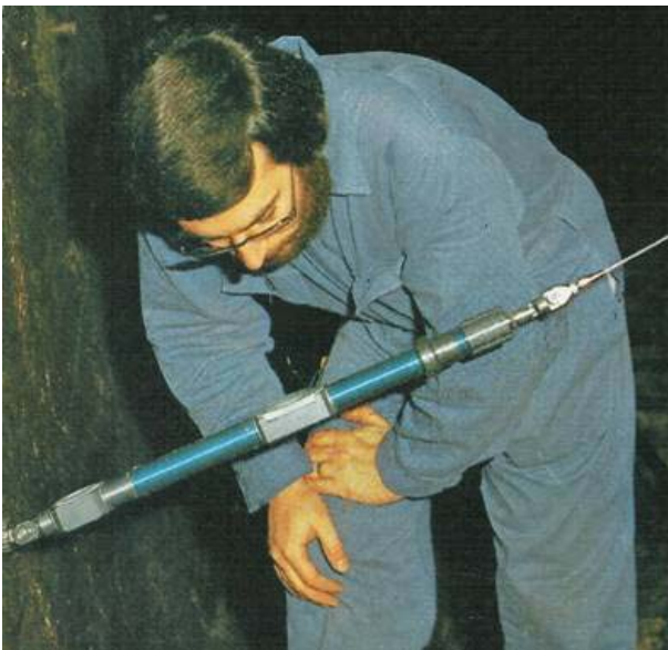
Figur 2.13-1: Distometer in Messposition
